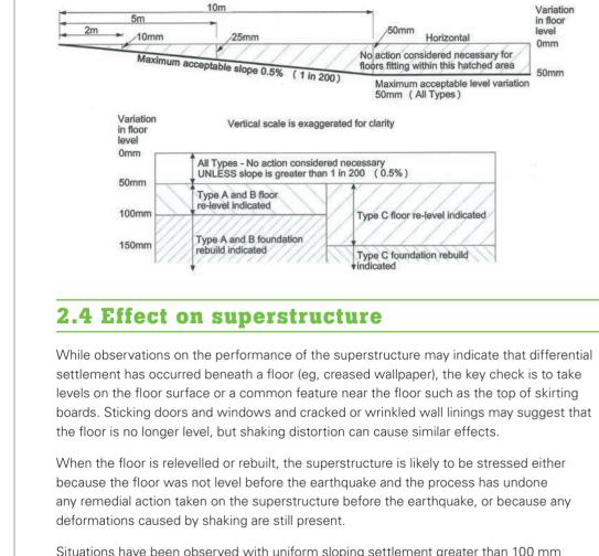
*Figure 2.2: Diagrammatic representations of slope and overall variation limits from Table 2.3*
