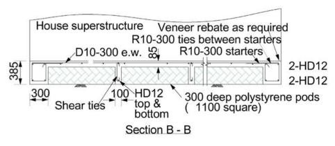
The ground immediately beneath the polystyrene and ribs must have a minimum geotechnical ultimate bearing strength of 200 kPa, or the system should be subject to specific engineering design (refer to section 3.4.1). Shear ties in accordance with NZS 3101 are required in the ribs.
