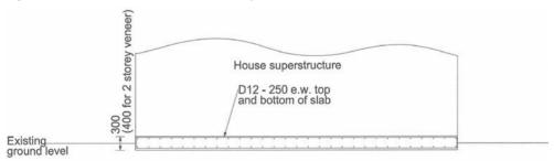
Note: NZS ground clearances adjacent to house foundation must be complied with. DPC omitted for clarity.
