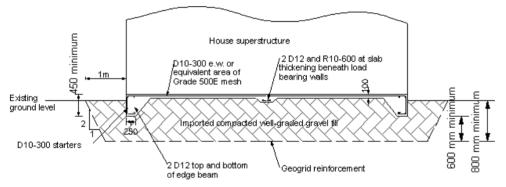
**Option 2** – Construct a thick slab foundation over the existing soil.
