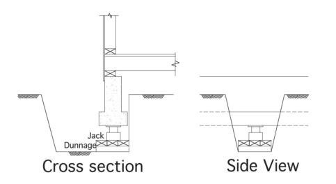
Foundation relevelling involves excavating pits at discrete locations to the perimeter of the foundation wall, and installing jacks in each pit to the underside of the wall to raise it to the correct level. With the foundation repositioned, flowable grout is introduced to the cavity created under the raised foundation. Once the grout is cured, the jacks are removed and the pits refilled.
